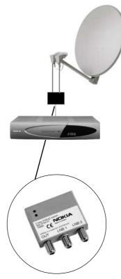
DiSEqC switch with 2 inputs
